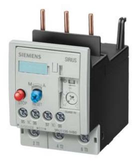
OVERLOAD RELAY, 5.5...8 A, 1NO+1NC, SIZE S2, CLASS 10, FOR CONTACTOR MOUNTING
