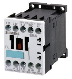
CONTACTOR, AC-3 3 KW/400 V, 1 NC, AC 110V 50HZ/ 120V 60HZ 3-POLE, SIZE S00, SCREW CONNECTION
